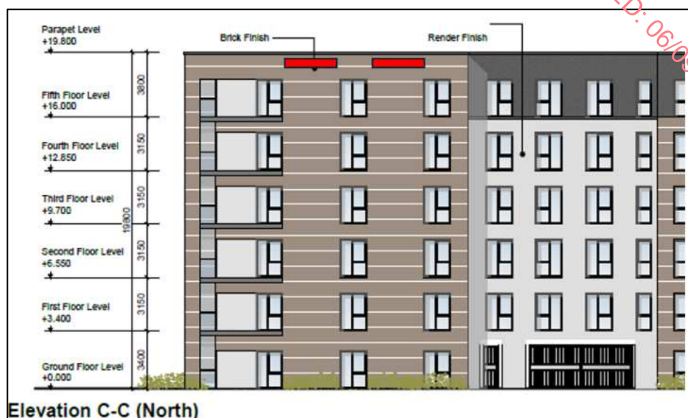
Figure 8-16 Examples of suitable locations for Swift Bricks on Block A (northern elevation) shown in red (adapted from MCORM Drwg: PL207).
