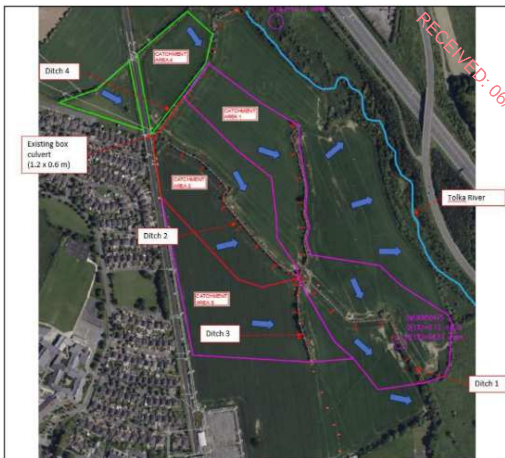
Figure 8-3 Existing drainage ditches across the Site and surrounding lands (source: ESR (DBFL, 2024))
